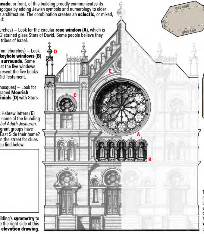
This masonry building uses arches above the windows to frame and support the openings. Cut out, fold, and glue the template above to build one of these wedge-shaped stones. You can trace and assemble this voussoir six more times to create a complete arch, as seen in the diagram.
